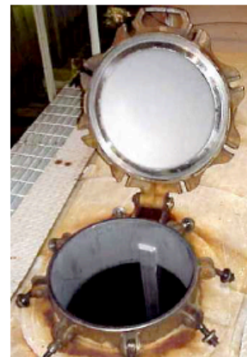
FIGURE 1: GENERAL PURPOSE RAILROAD TANKCAR MANWAY
